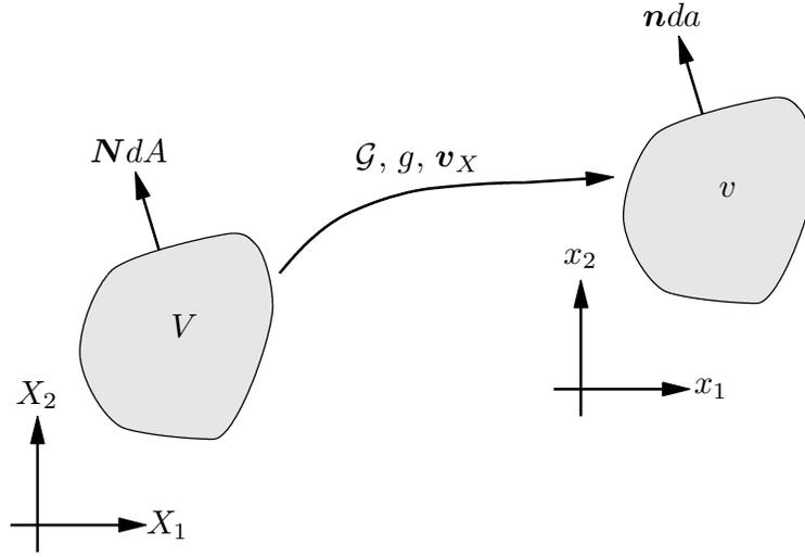
Figure 1. Mapping between the physical and the reference domains.
