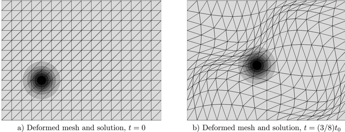
**Figure 3. Meshes and solutions for initial conditions (a) and at time  $t = (3/8)t_0$  (b). Note that the deformed mesh is used only for visualization, the calculations are done in the reference space using mapped equations.**
