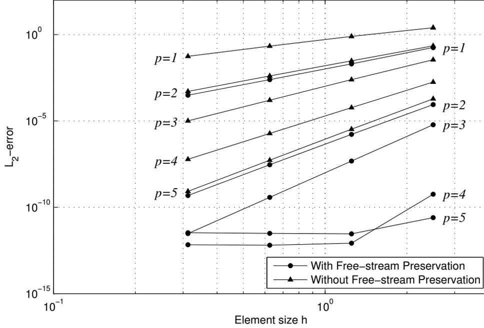
Figure 5. The convergence of a pure free-stream problem with and without the free-stream preservation technique.
