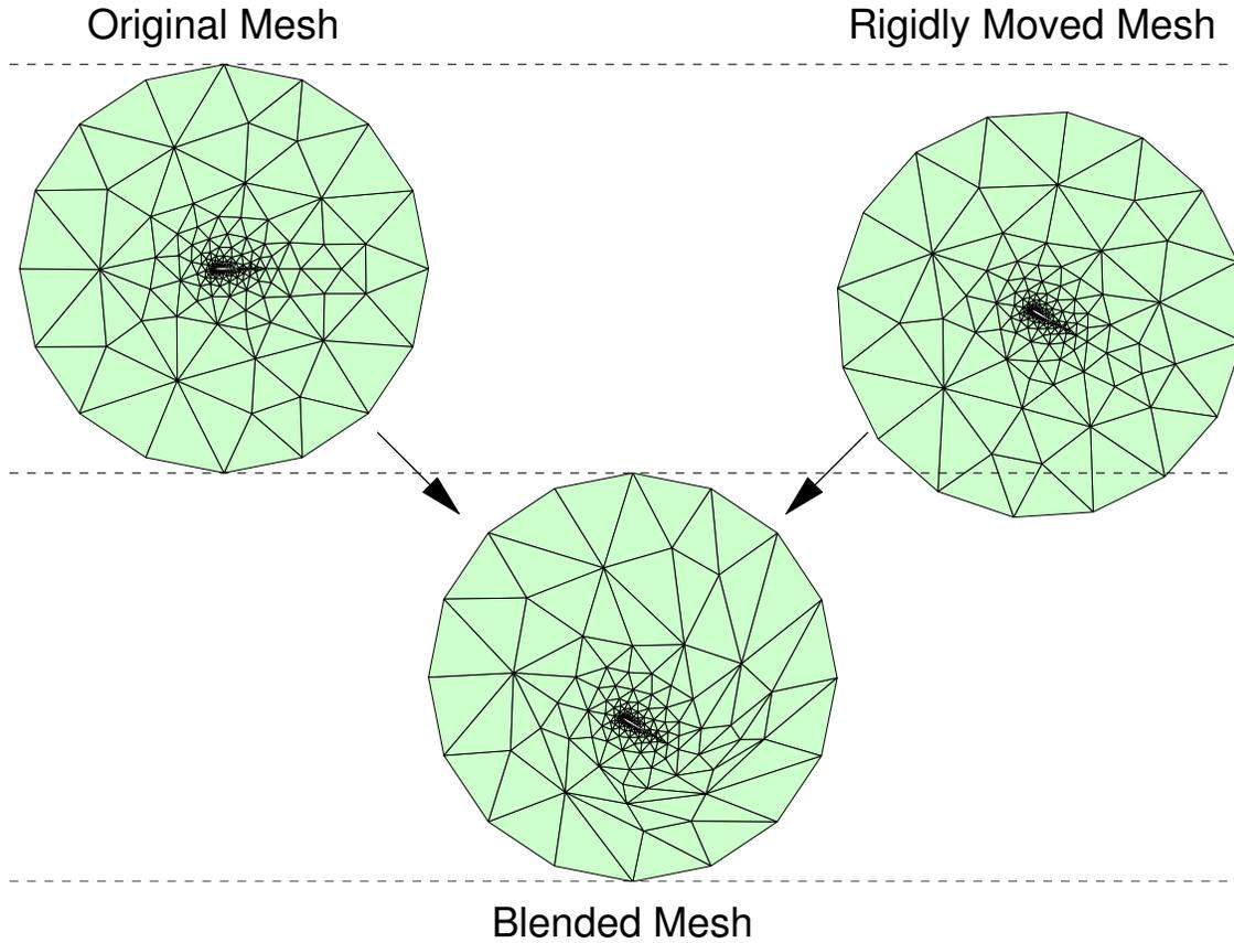
Figure 2. Deformation of a domain by blending of two rigid displacements.
