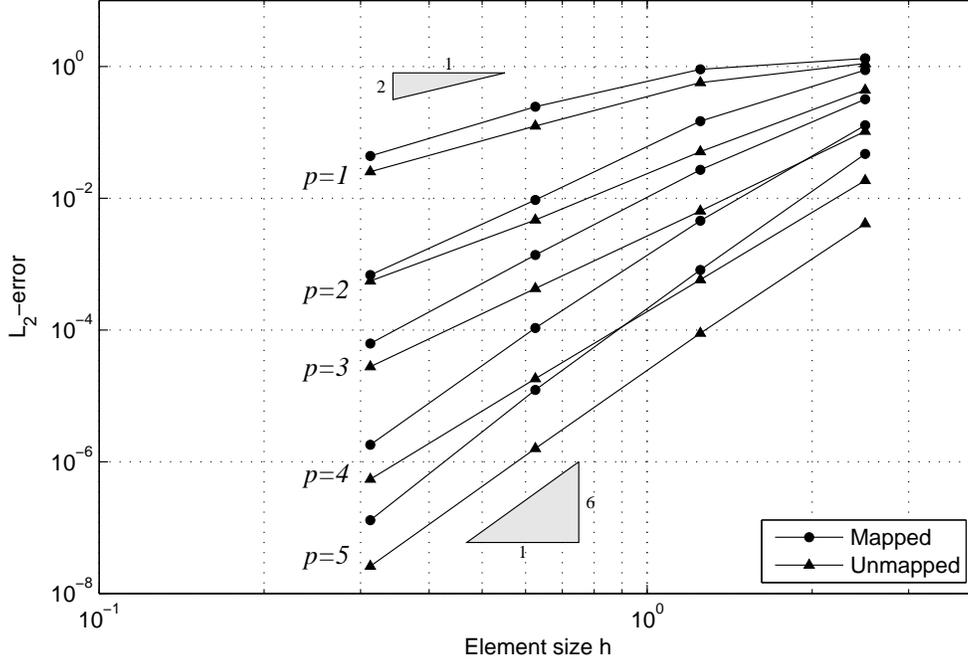
Figure 4. The convergence of the mapped and the unmapped schemes for the Euler vortex problem. Three mesh sizes are used and polynomial orders  $p = 1$  to  $p = 5$ . The optimal convergence  $h^{p+1}$  is achieved in all the cases, although the constant is larger for the mapped cases because of the non-uniform resolution of the vortex.
