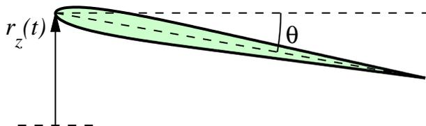
Figure 8. The pitching airfoil model.
