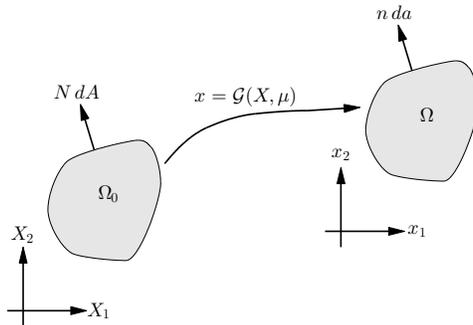
Figure 1: Mapping between reference and physical domains.
