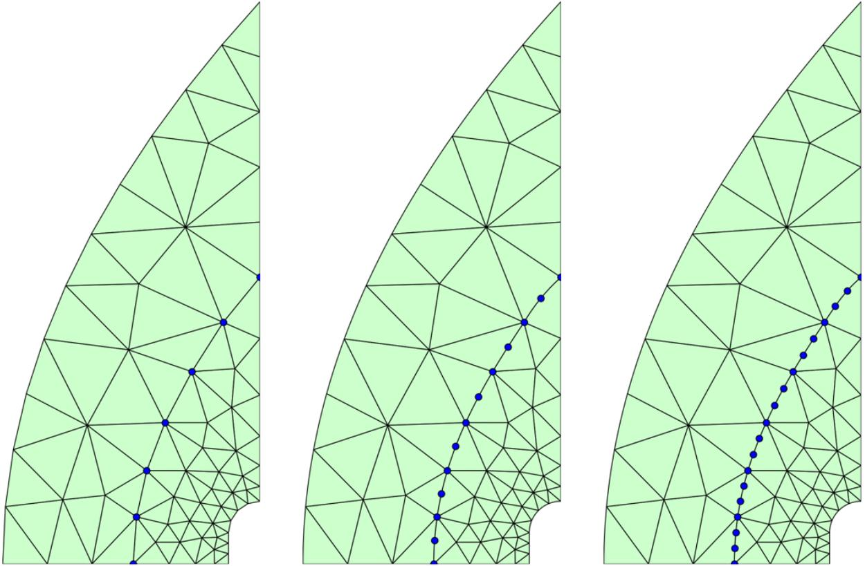
Figure 4: Reference domain and mesh with  $|\mathcal{E}_{h,p}| = 102$  elements and polynomial orders  $p = 1$  (left),  $p = 2$  (center),  $p = 3$  (right). The blue circles identify parametrized nodes, i.e., nodal positions that whose displacements compose the optimization variables  $\phi$ . Only the displacement normal to the boundary are taken as optimization variables for the two parametrized nodes that lie on boundaries.
