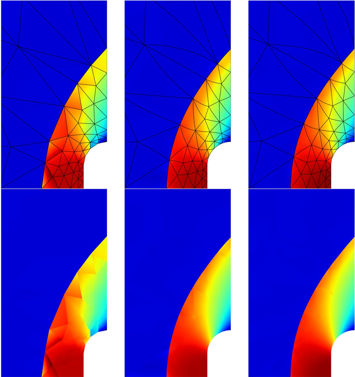
Figure 5: Solution of two-dimensional Euler equations (density) with supersonic inflow  $M = 4$  using discontinuity-tracking framework with polynomial orders  $p = 1$  (*left*),  $p = 2$  (*center*),  $p = 3$  (*right*). The deformed mesh provided by the tracking framework is included in the *top row* to show the high-quality curved elements that track the shock location. The mesh is not included in the *bottom row* to clearly show the solution features away from the shock.
